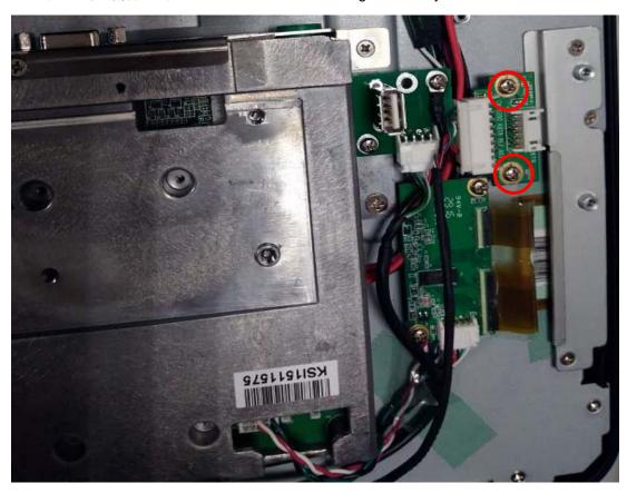
11.连接模块的 MSR cable 线从上部走 Assembly the board to here, and put the cable in order, like the below picture.
