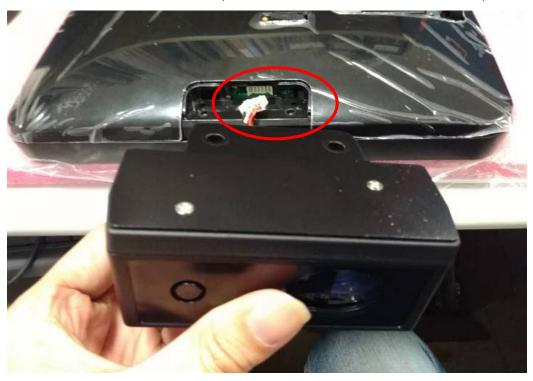
14 用 2 颗螺丝,锁在以下位置 (Install it to the following location by 2 screws)
