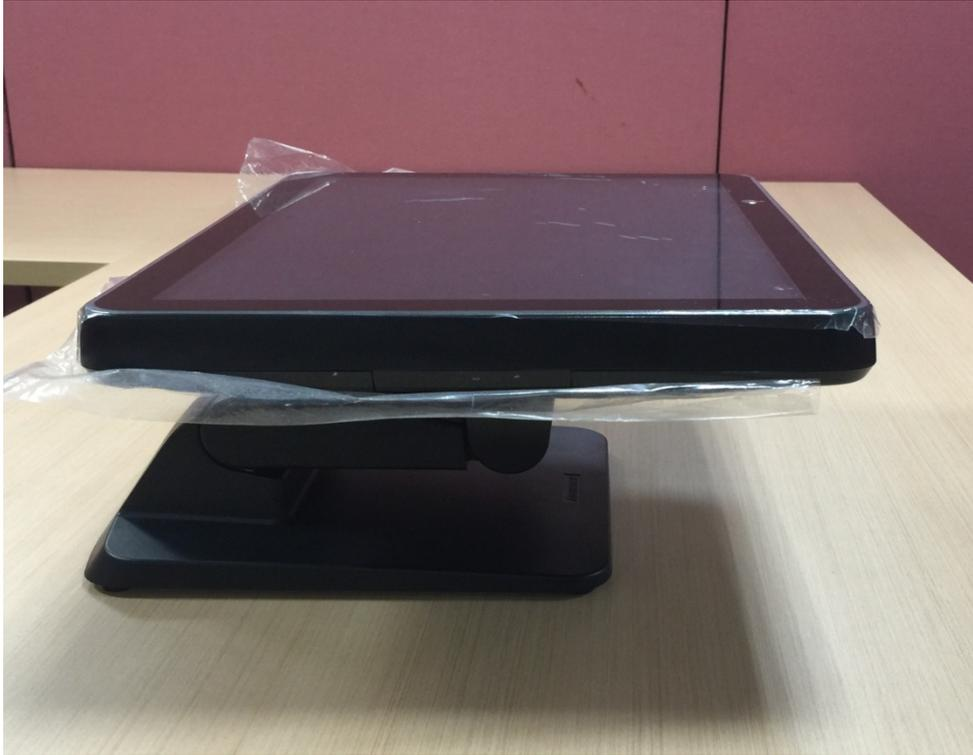
2. Adjust the 1<sup>st</sup> hinge on stand base. Use left hand to press the stand base, and push the screen to the highest position (~ 60°) by your right hand.
