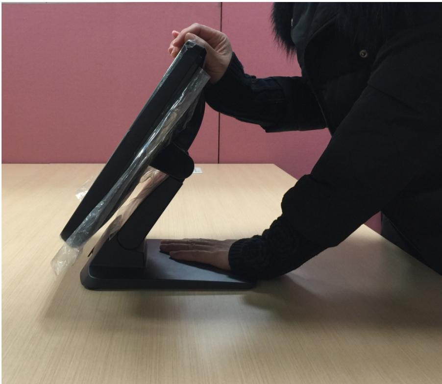
3. Adjust the 2<sup>nd</sup> hinge on screen. Use left hand to press the neck of the stand, adjust the screen by your right hand. Adjust the screen angle to the best comfortable viewing experience.
