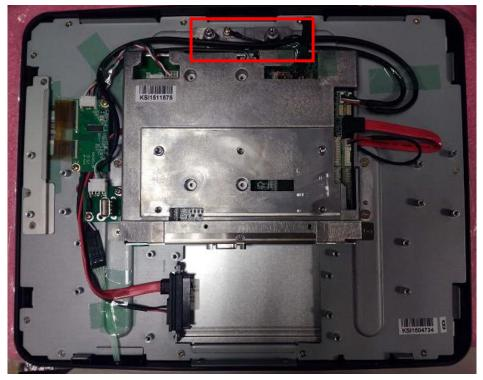
10. Take out the 7" monitor. It is with the rear mount bracket & USB cable.
