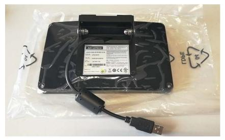
11. Assembly 7" monitor to the red block area, via 2 screws, then connect the USB cable on 7" monitor to the USB port.
