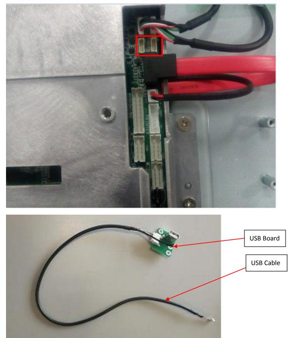
9. Assembly the USB board to below location. Then assembly all the parts back.
